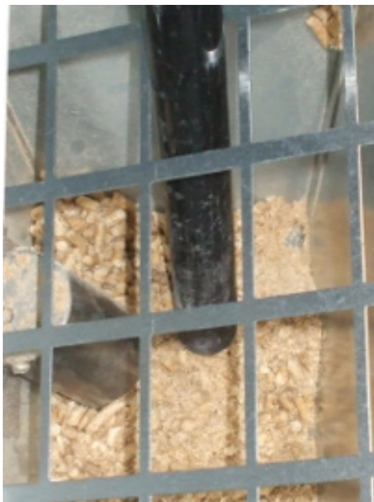
Fig. 31 - Hopper and auger cleaning
